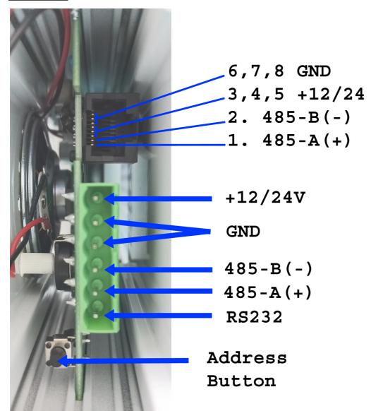
Note that matching connections shown are physically connected between the jack and the green header. So if the last display on a run is connected via the modular jack, then the  $120\Omega$  terminating resistor may be fitted to this units green terminal block.
